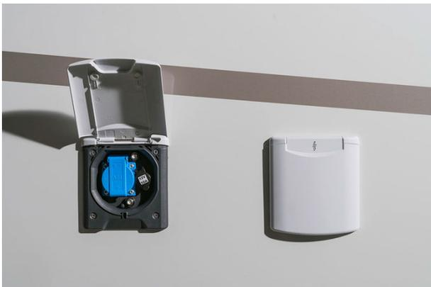
The optional universal awning socket with 230 V, 12 V and TV connections can even be used to hook up and supply power to electrical equipment outside the caravan.
