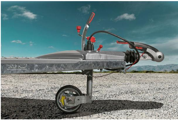
The premium drawbar jockey wheel with integrated load indicator, comfort wheel and integrated swing arm suspension is available as an option for the ERIBA Nova SL.
