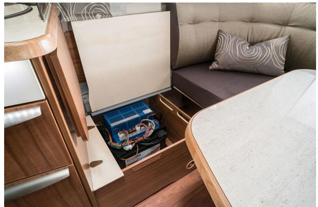
The electro-autonomy package, which is available as an optional extra, consists of a 95 Ah AGM living area battery, a 230 V automatic charger, an LED charger control display and a booster. It is housed in the storage box underneath the seating area.
